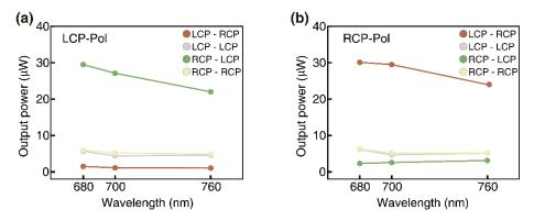
Fig. S7 Circular polarization resolved transmission efficiency of the metasurface holograms. (a) Measured spectra of the LCP-Pol metasurface hologram. (b) Measured spectra of the RCP-Pol metasurface hologram. The incident light has a power of  $100 \mu$ W.
