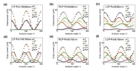
**Fig. S2** Experimental results for retrieving the Jones matrix of the linear and circular metasurface polarizers. (a)–(f) Experimental results corresponding to the LP-Pol-H, RCP-Pol and LCP-Pol working at different wavelengths. The six kinds of incident polarization states include H, 45°, V, 135°, LCP and RCP.
