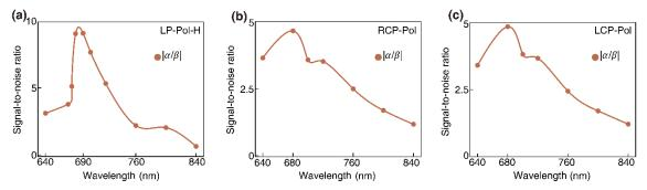
**Fig. S3** The spectra of Jones matrix's signal-to-noise ratio of the metasurface polarizers. (a)–(c) Measured spectra of LP-Pol-H, RCP-Pol and LCP-Pol.
